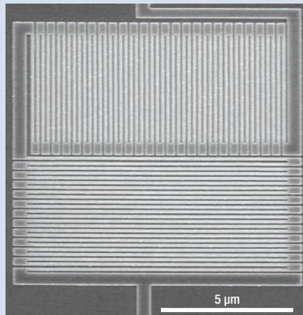
The detector has a fill fraction of 50% and an active area of  $10\ \mu\text{m} \times 10\ \mu\text{m}$ . The result is identical quantum efficiency for all polarization directions.
