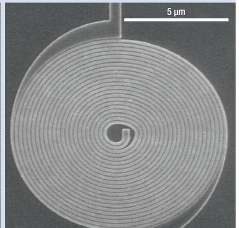
for this geometry; the diameter of the spiralling detector is  $10\ \mu\text{m}$ .
