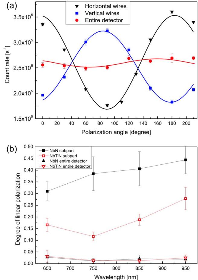
FIG. 2. (Color online) (a) Count rate versus polarization angle for the perpendicular detector made of NbN. The laser spot (wavelength 650 nm) is focused on respectively the horizontal wires (red triangles), the vertical wires (green squares) and the entire detector (orange circles). (b) Degree of polarization versus wavelength for the perpendicular detectors, made of NbN and NbTiN, with one sub-part (squares) or the entire detector (triangles) illuminated.
