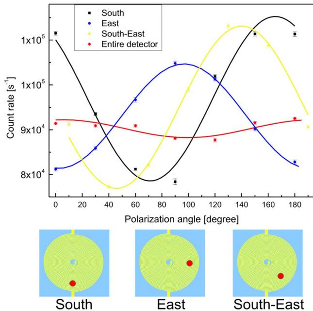
FIG. 3. (Color online) Polarization dependent count rate for a spiraling SSPD. The laser spot (wavelength 650 nm, diameter  $1\ \mu\text{m}$ ) is focused on different regions of the detector (indicated in the lower part). When the entire active area is illuminated uniformly, the count rate exhibits almost no polarization dependence (red curve).
